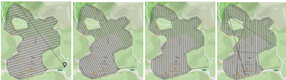
Figure 12 Compared path planning methods - from left to right: Our method, Brute force, Single orientation, Boustrophedon decomposition + Brute force
