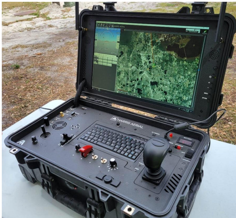
Figure 4 Real example of a GCS (source: https://hse-uav.com/ )
