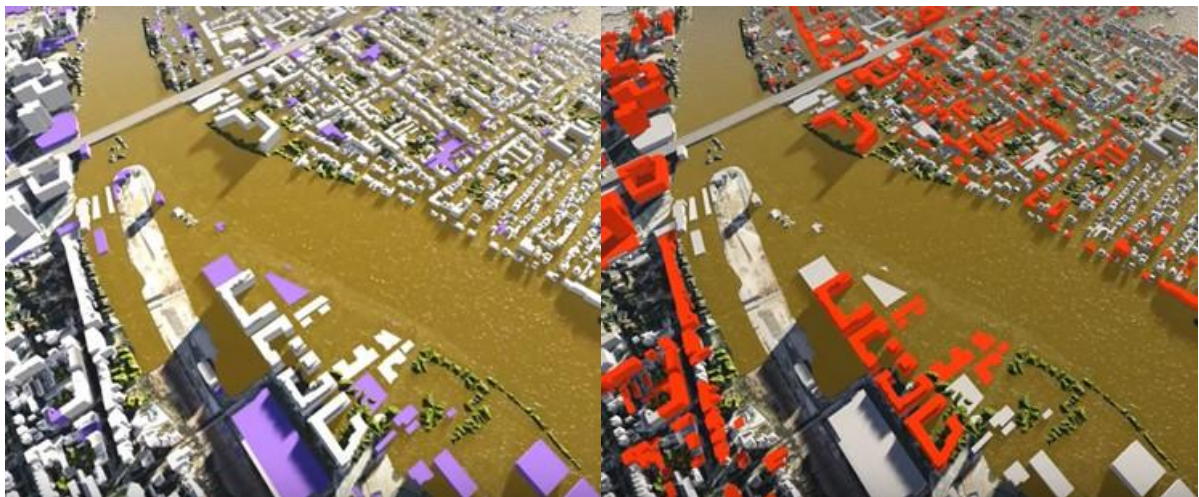
Figure 24: Screening of infrastructures according to their criticality for the community and their exposure to the crisis effect
